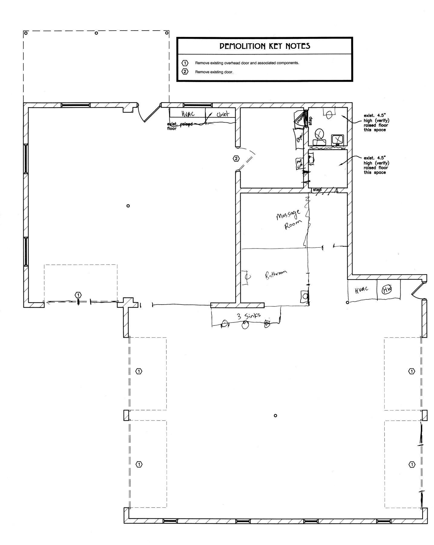
EXISTING CONDITIONS / DEMOLITION FLOOR PLAN
