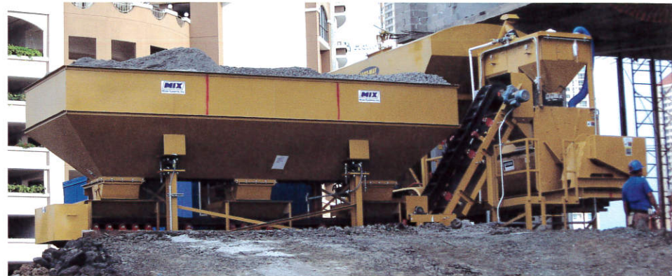
Mark IV Skid Mount with Model 54 Praschak™ Horizontal Shaft Mixer on high-rise construction site; 230 yds./day output.
