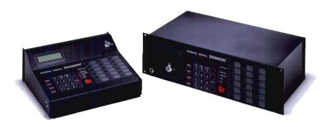
Federal Signal's SS2000 encoder is a versatile, user-friendly control unit. Available in one-way control and two-way status monitoring, the controller is offered in DTMF or FSK formats. Encoded command sequences are field programmable and stored in memory for retention even when electrical power is removed. Federal Signal's SSLOADER offers an easy Windows-based software package for configuring the encoder's command sequences and operating parameters.
