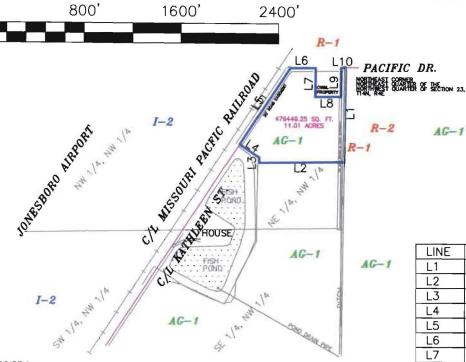
LINE BEARING DISTANCE S 00°35'43" 776.63 L1 W S 89°13'34" L2 W 703.50' 00'35'43" L3 43.60 N 56'35'53" W L4 193.86 N 33°24'08" L5 E 754.15 89'13'34 L6 N 209.03 S 00°35'43" W L7 238.72 L8 N 89'13'34" Ε 208.72 N 00°35'43" L9 238.72 N 89°13'34" L10 E 40.01
