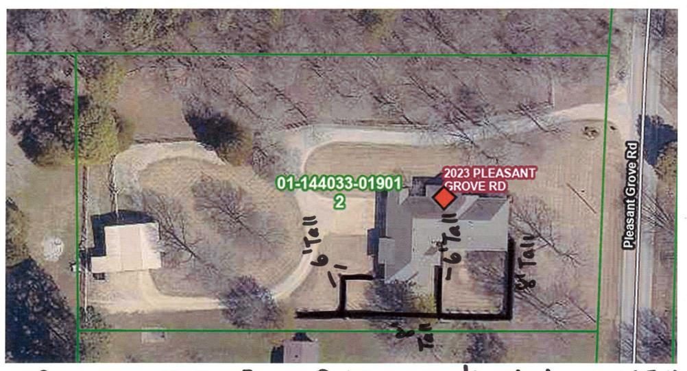
Replacing 8' Tall Fence, Brick posts will not change 10' Tall Inner Fence 6' Tall Be placement
