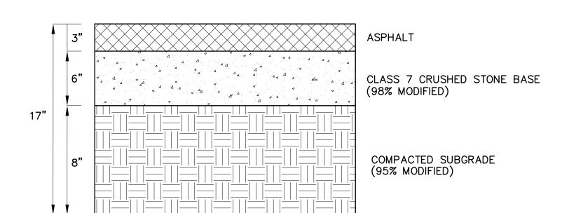
6 TYPICAL ASPHALT PAVING DETAIL
