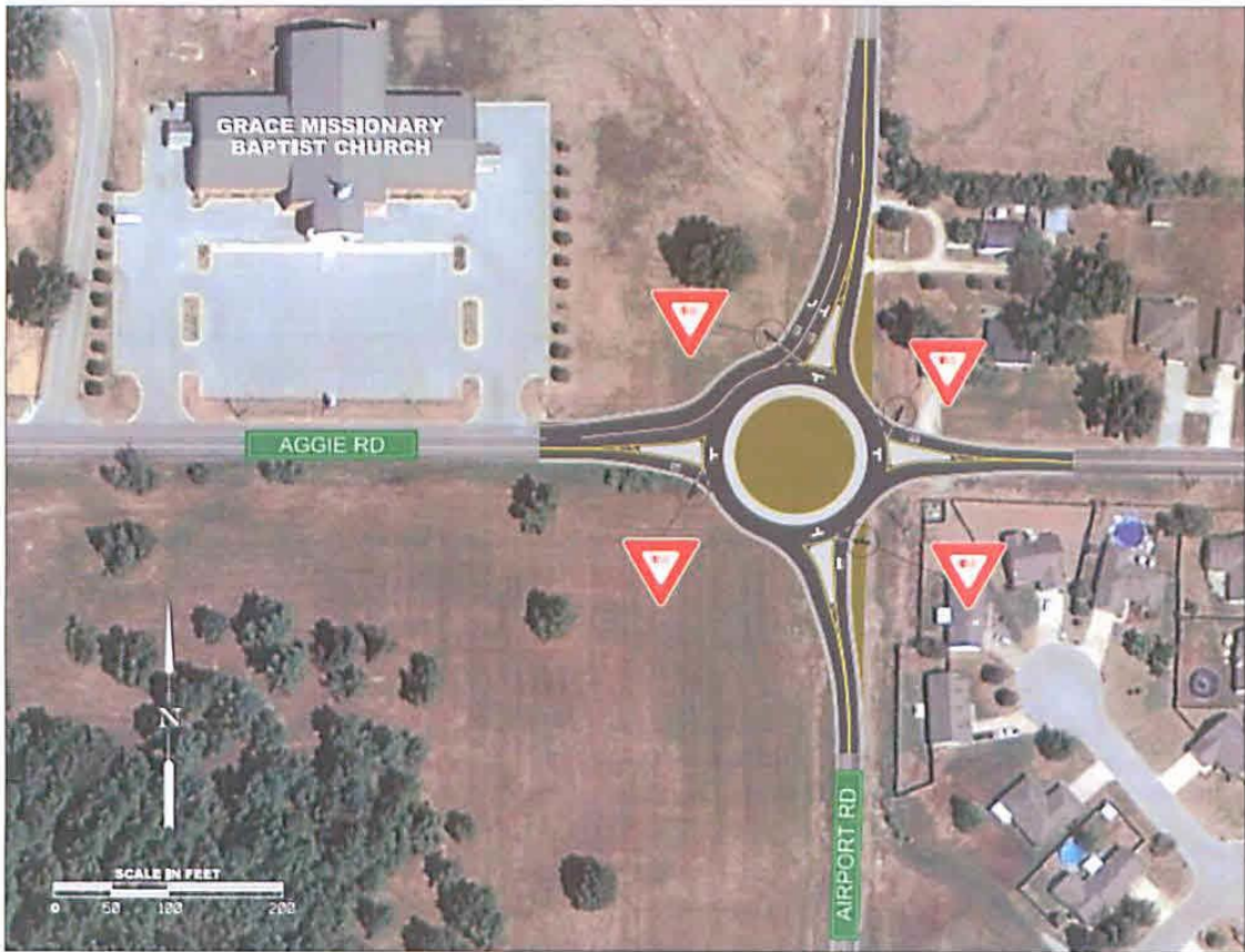
Figure 2: Conceptual Layout of Proposed Roundabout: Hwy. 351 and Aggie Road Intersection Source: Garver, LLC. January 2014
