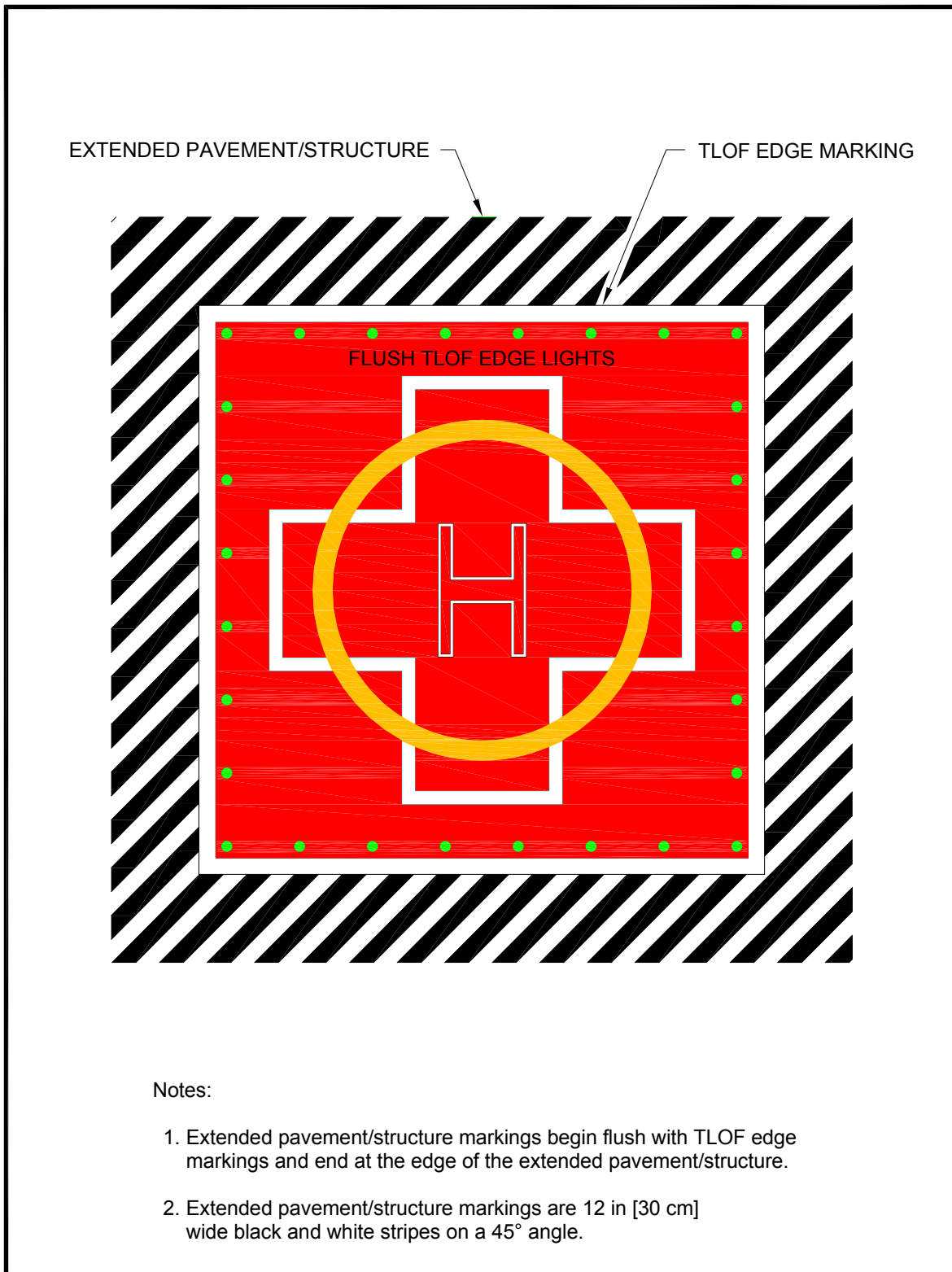
Figure 4–26. Extended Pavement or Structure Marking: Hospital
