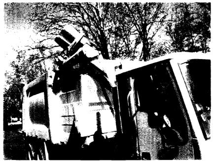
Automated trucks picks up residential houses in Jonesboro, these trucks average between 1,200 to 1,500 daily picks up a week. They are the bulk of operation; it is a one man operation and as you can see the driver controls the arm from inside the cab they pick up the container and empty it into a hopper; if containers are too full or trash isn't bagged it can cause a huge mess.
