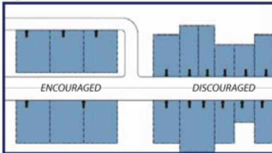
Internal roads provide access to multiple lots with minimum curb cuts on the adjacent road.
