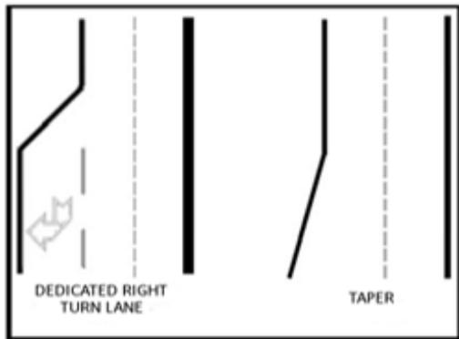
The length of this lane will vary according to the speed of traffic on the roadway and expected traffic volumes. However, the lane or taper should be of sufficient length so as to allow the turning vehicle to leave the through lane at the posted speed limit, decelerate, and negotiate the turn.
