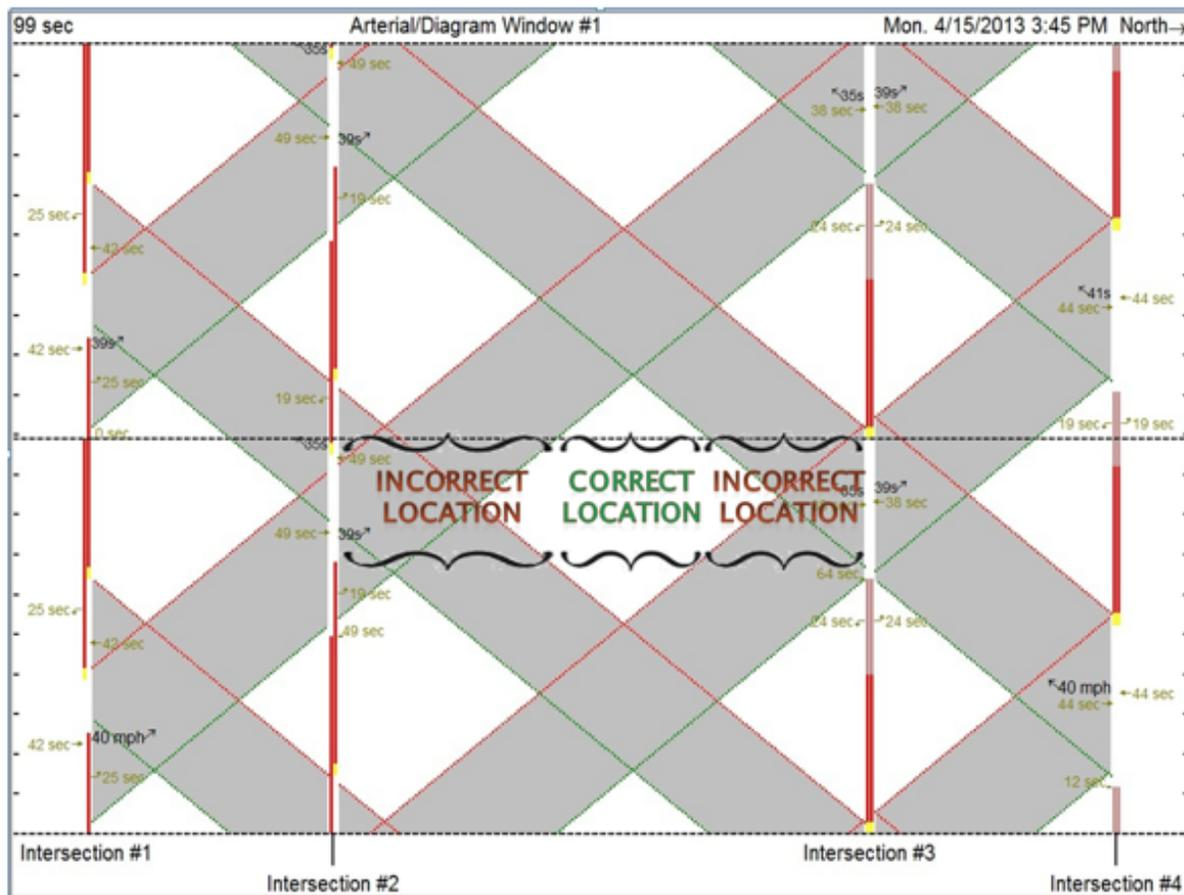
**Figure 6.1: Traffic Signal Location Selection
