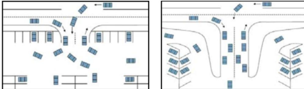
Insufficient throat length and poor site planning can result in unsafe conditions and may result in vehicles queuing, or stacking, in the roadway, interrupting traffic flow.
