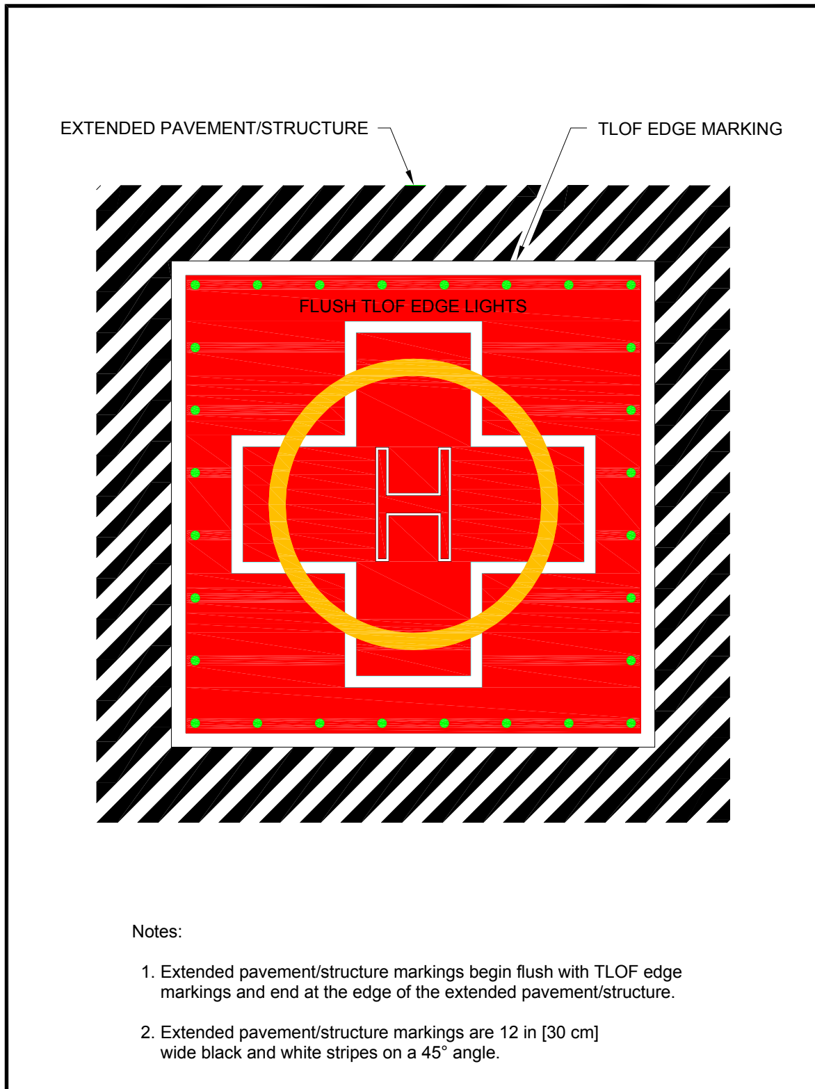
Figure 4–26. Extended Pavement or Structure Marking: Hospital
