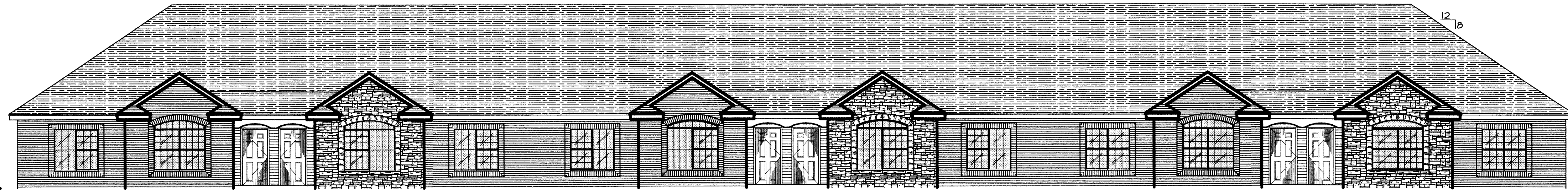
BLDG "B" - SIX PLEX FRONT ELEVATION 1/8"
